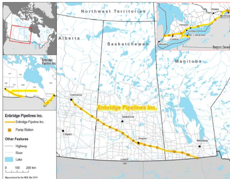
The Enbridge pipeline system, shown in Figure 1, is 7,747.04 km of oil pipelines that extend from Edmonton, Alberta, to Montréal, Québec, connecting with other oil pipelines in the United States at the Manitoba/North Dakota and Michigan/Sarnia Ontario borders.
